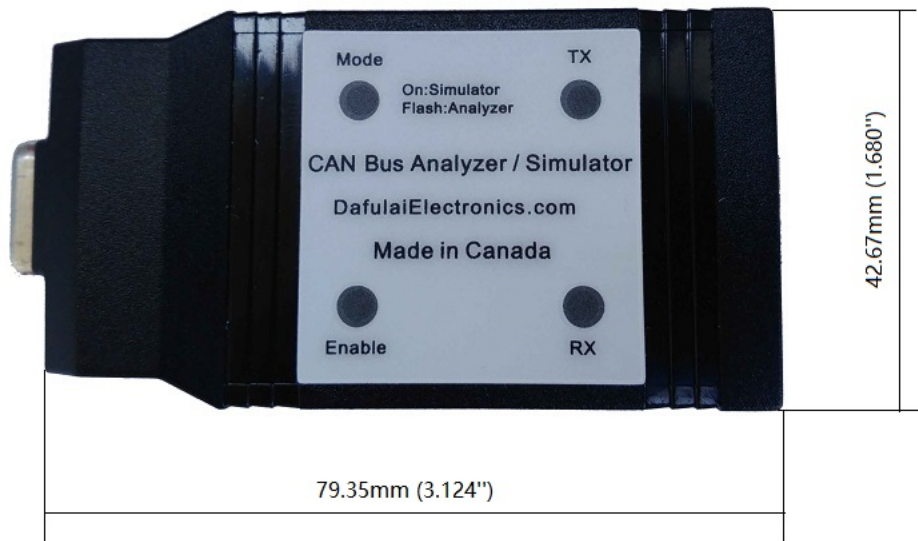
Fig.1 Hardware of CAN Bus Analyzer
