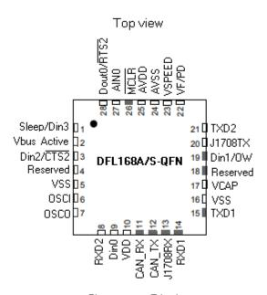
Pins are up to 5V tolerant
